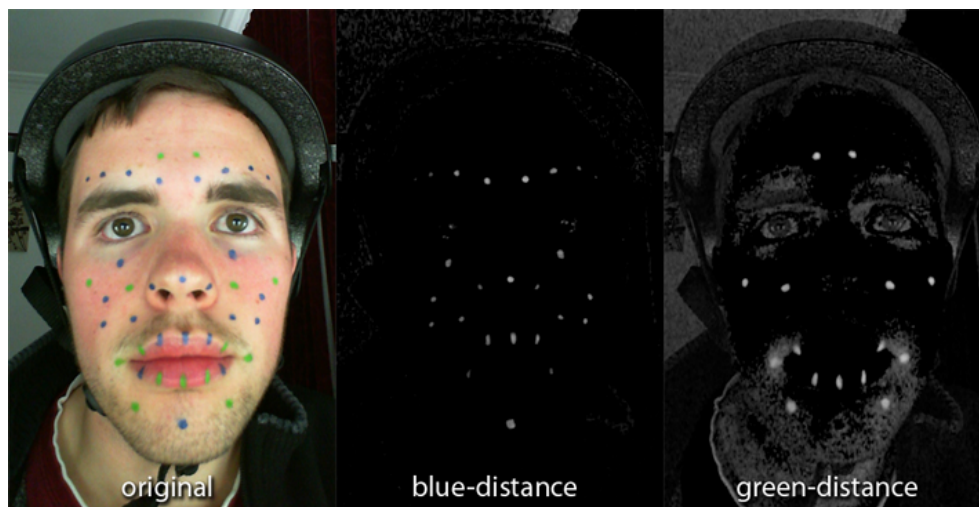
Figure 2: The results of applying the blue and green distance calculations to an original video frame.
