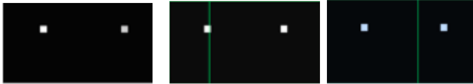
Figure 5 Median cut and Variance cut (the middle one shows that median cut may behave improperly when two bright light are placed in the same region) [9,10]
