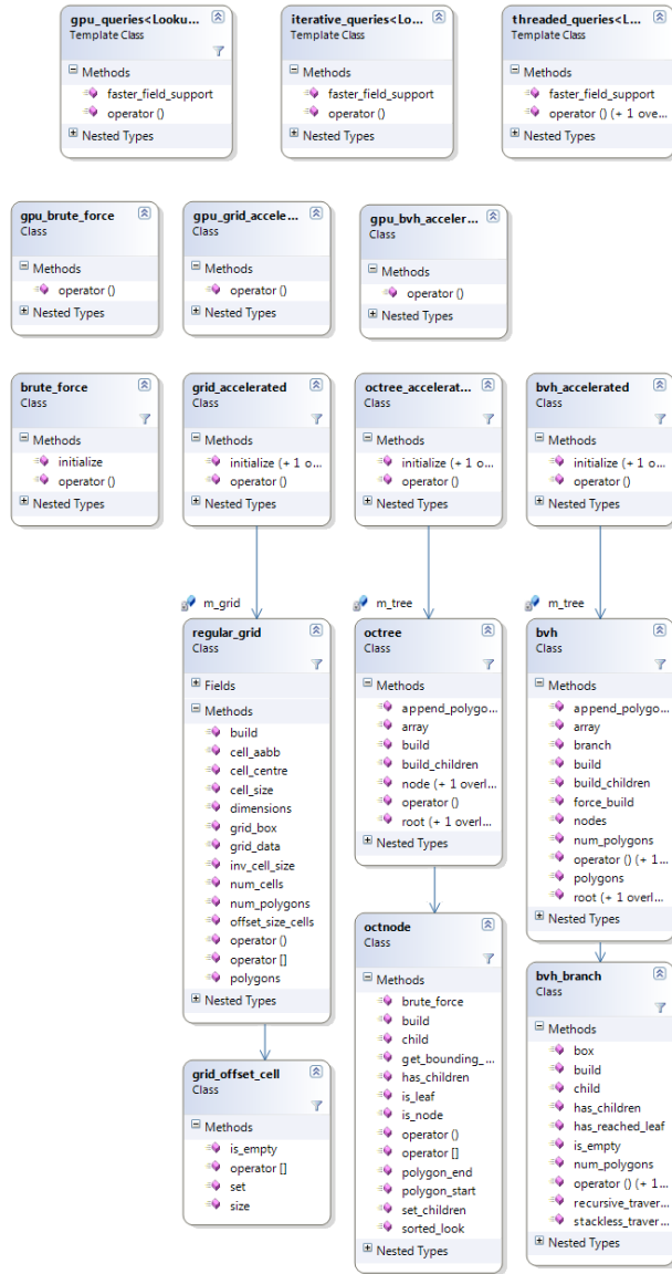
Figure 6.2: The UML diagram of the look-up policies and multiple queries policies
