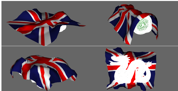
Figure 5.21: Cloth colliding with the Buddha (100 000 faces) and the Stanford Dragon (100 000 faces) in real-time
