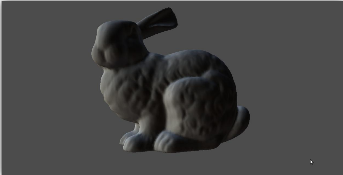
Figure 4.2: Rendering example: The Stanford Bunny lit by spherical harmonics based lighting. The light probe used is Paul Debevec's "beach_cross". 100000 samples and 3 bands were used.
