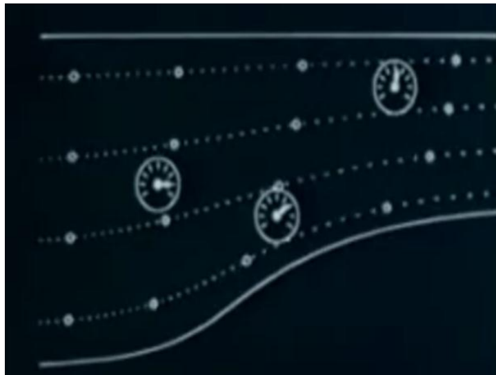
Figure 1 : Eulerian Particles Passing through fixed points in space (by the National Committee for Fluid Mechanics)
