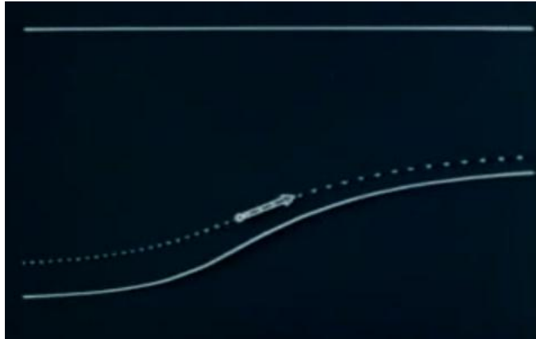
Figure 2 : Lagrangian Particle moving through space and time with a velocity vector attached to it. (by the National Committee for Fluid Mechanics)
