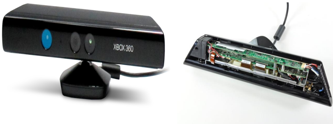
Figure 2 Illustrating the Xbox 360 kinect and its inside containing the SOC processor [geek.com, 2013]
