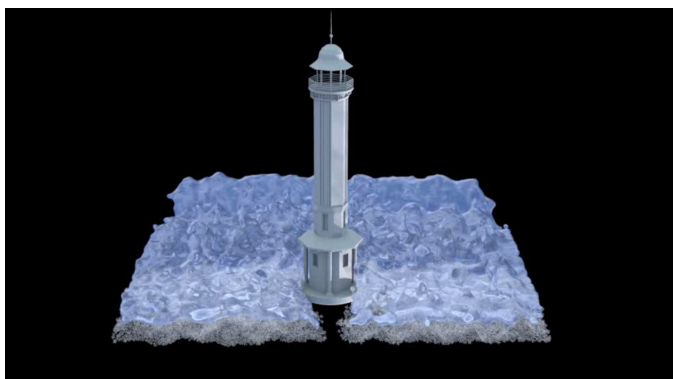
Figure 4.7: The lighthouse test. When the fluid collides with the solid object, the velocities are changed and result to move around it
