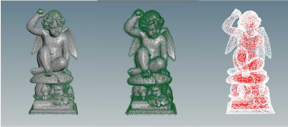
Figure 23: (From left) Normal inversion for the geometry ( .bgeo ): model with inverted normals, model with fixed normals and model with aggregation applied
