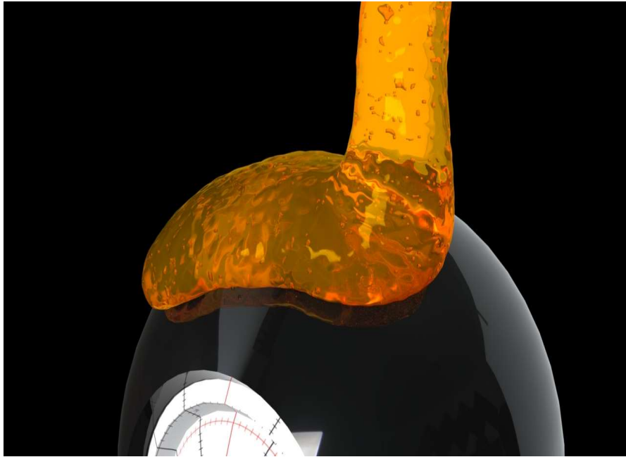
Fig 3. Simulation Parameter: Particle separation : 0.003, Thin sheet point count: 0, Thin sheet distance :0, Thin sheet max vel : 0, Thin sheet scale: 120, Viscosity : 75, Min age: 0.6, Liquidity : 40, Solidity: 60, Drag :0.001, with Detailing and Reseeding features On.
