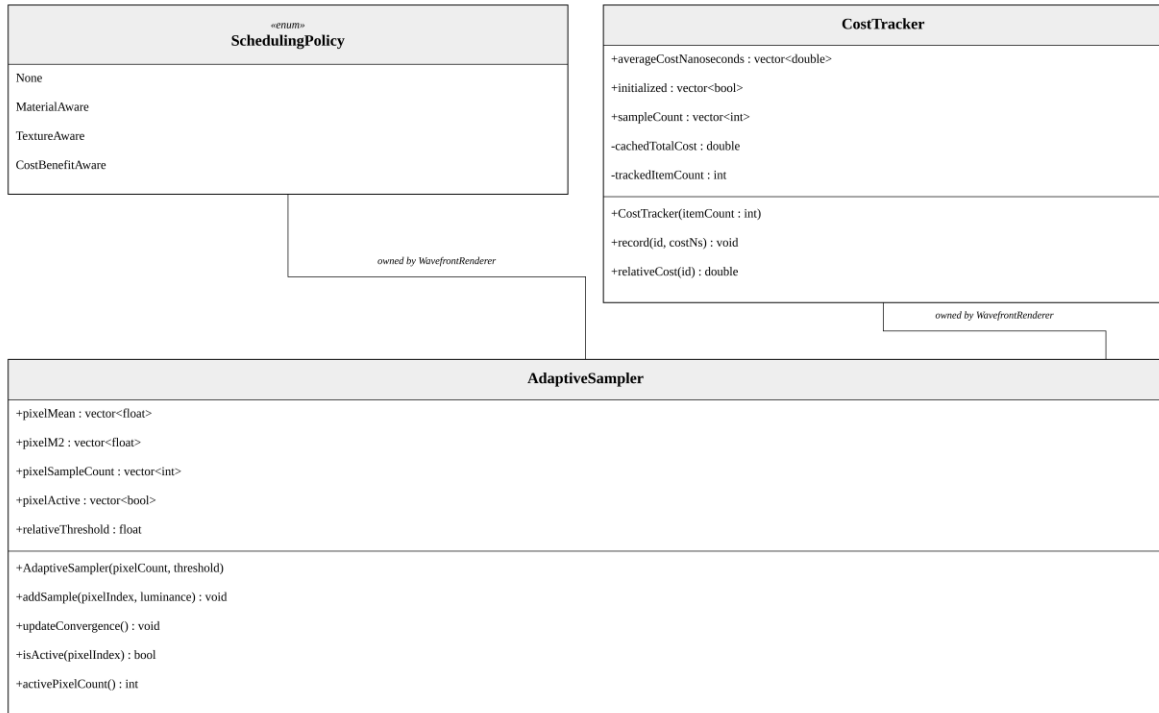
Figure A. 8 Scheduling policies, runtime cost tracking, and adaptive sampling components.
