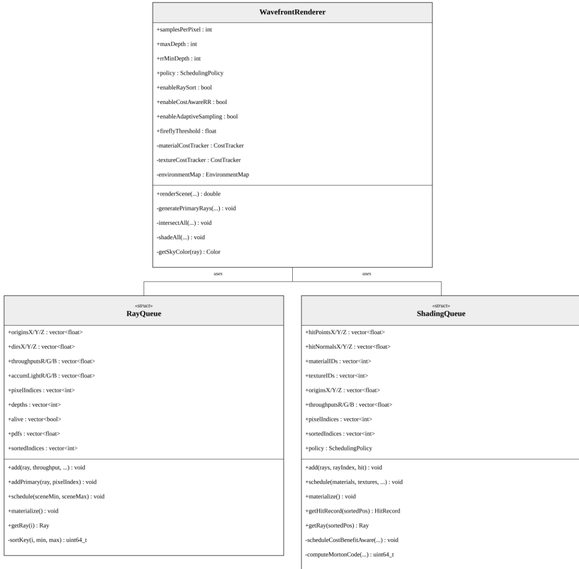
Figure A. 7 Class structure of the WavefrontRenderer, RayQueue, and ShadingQueue.
