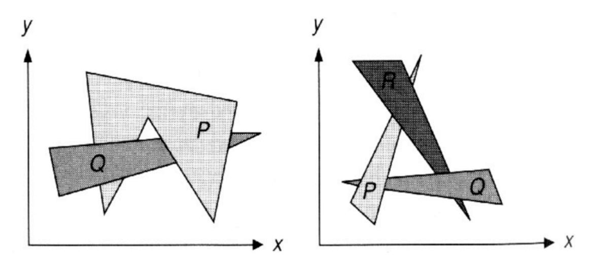
In these cases, the algorithm splits the polygon faces down further so that a linear order can be generated.
